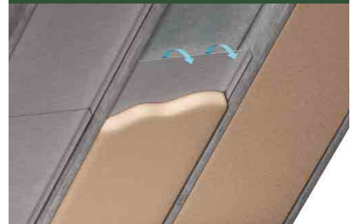
✓ Pitched roofs with ventilation layers
